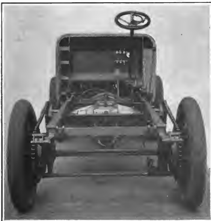
REAR END OF DAIMLER CHASSIS, SHOWING CHAIN DRIVE.
